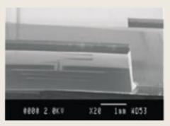
Figure 1: Membrane supported Yagi Uda antenna membrane obtained by silicon micromachining – (common work of IMT and LAAS-CNRS Toulouse).
